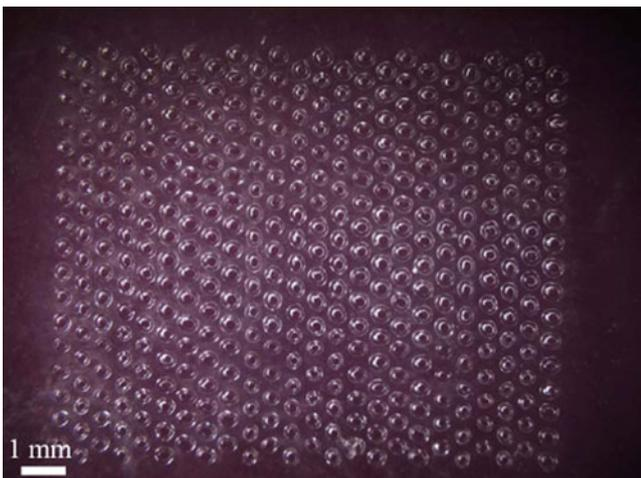
**Fig. 1** Mask used to selectively expose areas of skin to microdermabrasion. The 408 approximately circular holes of 125  $\mu\text{m}$  diameter were drilled into the polymer mask using a CO<sub>2</sub> laser. The mask was adhered to the skin with tape, and the microdermabrasion tip was moved across the surface of the mask to abrade the skin exposed through the holes.
