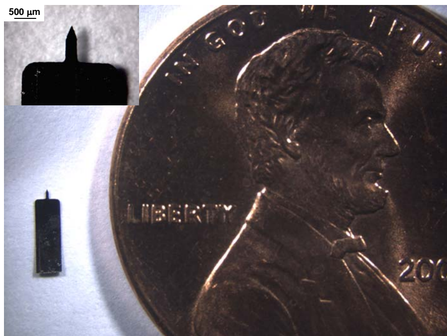
Figure 4.2.1. Bright field microscopy image of a single solid stainless steel microneedle used in in vivo insertion experiments shown next to a penny. A close view of the needle, which is 500 \mu\text{m} in length and 45^\circ in tip angle, is shown at the upper left corner of the figure
